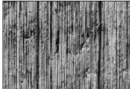
Microscopic view of mechanically polished surface with grit 400 Ra 0,25 \mu\text{m} / 10 \mu\text{-inch}
